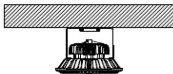
Diagram3: Fix the U bracket to the wall by nut,plain cushion, Spring shim
