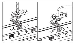
6.Place all connections and exposed wire inside of fixture and reattach power access plate.
