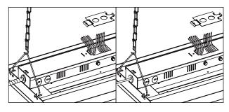
5.Connect the green (ground), black (line) and white (neutral) wires of the AC line to the similarly colored wires of the fixture's power supply using UL listed connectors. Place all connections and exposed wire inside of fixture and reattach power access plate.
