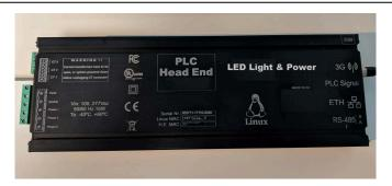
The Head End is installed in the electrical panel containing the circuits for the fixtures to be controlled. The Head End is responsible for managing each of the fixtures and sensors. It saves the configuration and time schedule of all fixtures, manages the network, and verifies the system is working properly.
